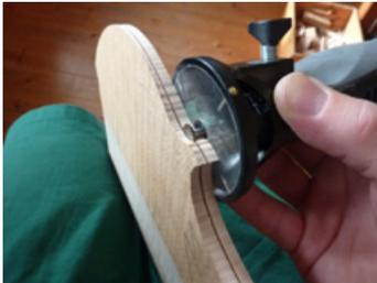
**2)** I use a small electric saw to cut the edge to the thickness of the finished corners and button. This saw can be used very precisely, owing to its small size and the large surface that rests against the plate. The thickness of the plate will depend on the depth of the fluting and the radius of the gouge — I generally cut it to 4.7mm.
