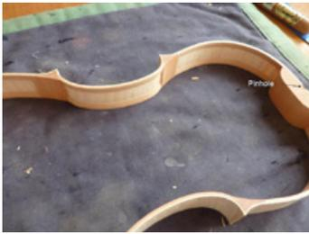
**1)** I begin with the outlines of the finished rib structure, with the linings in place on both sides. I transfer them to the back and front, including the desired overhang — initially this is 3.5mm, though when finished it will be 2.5mm. I try to use the middle seam as the centre line of the instrument because it plays an important part in the whole construction process.
