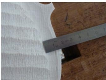
**3)** To begin the arching, I create a flat platform around 15mm from the edge for the bouts, and c.8mm for the C-bouts, using the saw cut as a guide. I then cut the provisional fluting, leaving an extra 0.2–0.3mm for security. The fluting goes all the way to the edge, leaving a margin of just 2mm. (I never need to measure this — fingertips or the presence of a good shadow are precise enough.)
