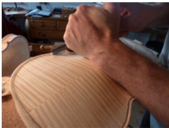
**9)** I cut the fluting almost all the way to the edge (leaving around 0.2mm) and cut down the purfling. Next, I work on the transitions to the arching and scrape arching. I scrape to the edge again (as described in step 4) without worrying about damage to the edge, as any mistakes will disappear when the edges are rolled over.
