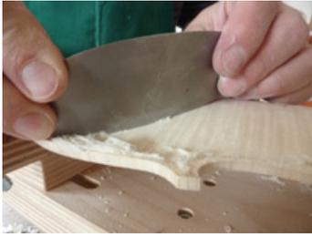
**4)** I connect the arching with the preliminary fluting and finish it. This step gives the arching the look of a classical model, but requires a little practice as the outlines and purfling are not yet finished. Scraping the arching right up to the edge creates a nice fluting and connecting area, which has a (naturel or unique) look. I am convinced of the historical validity of this step.
