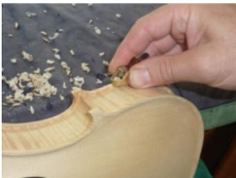
**7)** To finish off the outlines, I prefer to use a flat thumb plane for the bouts and a knife, plus a range of different files, for the inner curves.
